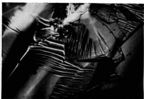
Fig. 1. Typical examples of Type II (hackle) structure in Samples A and B . 150 \times .
