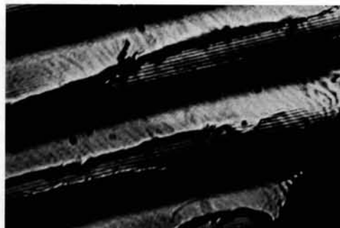
Fig. 5. An instance in which the optical effect is definitely associated with a lamellar substructure. 160 \times .
