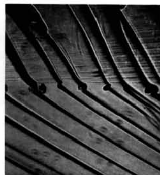
Fig. 8. Fractograph disclosing what appears to be the residua of a foreign phase (gas, liquid, or solid) which deposited during a certain period of crystal growth and later deflected the hackle cleavage traverse as shown. 160\times .
