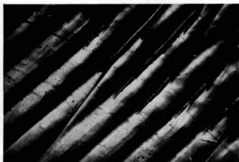
Fig. 2. Fractograph of an unusual undulating field in Sample A , showing an interesting relationship with the tip-ends of an intruding hackle structure. 80 \times .
